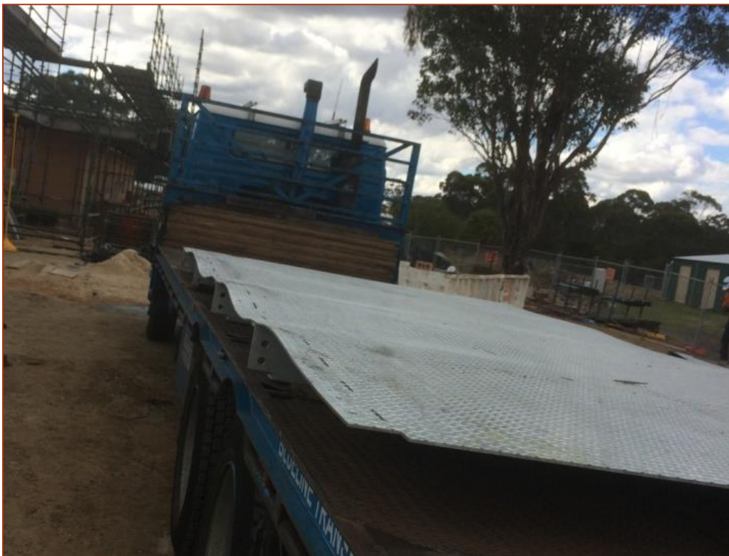
Figure 2: Distortion of a long, thin unbraced plate
