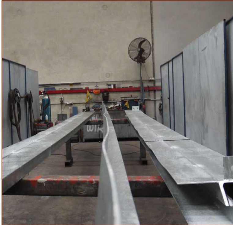
Figure 1: Variations in steel sections can lead to distortion of the differing attached sections
