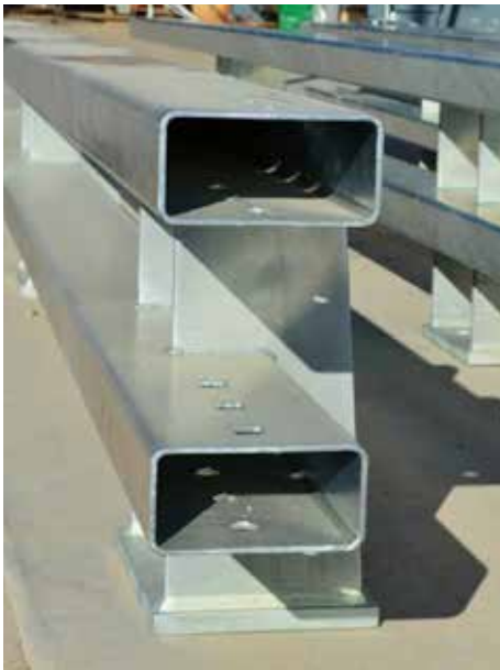
Only hot dip galvanizing can provide barrier protection to this bridge rail, inside and out.
